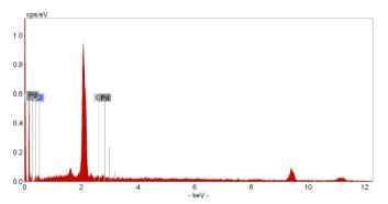
Fig. 2. EDS spectra of chitosan-based Pd (II) catalyst
