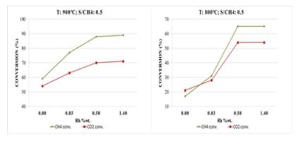
Fig. 1. CH4 and CO2 conversion as a function of the Rh content and reaction conditions
