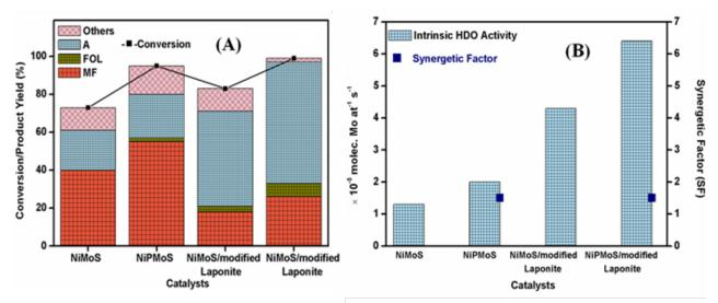
Figure (A) Conversion and Product yield of the catalysts, (B) Intrinsic HDO activity and synergetic factor of NiPMoS and NiPMoS/modified Laponite
