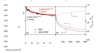
Figure 1. Comparison between REF and 3ALD-REF results and power fitting (a) / Extrapolation of fitted results to 8000 h operation (b).  $A = X(\%) \cdot GHSV/100$
