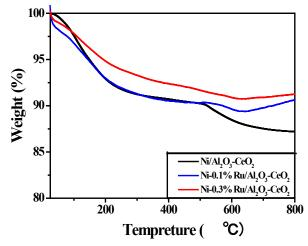
Fig2. TG profiles of the spent catalysts after 6 h reaction.
