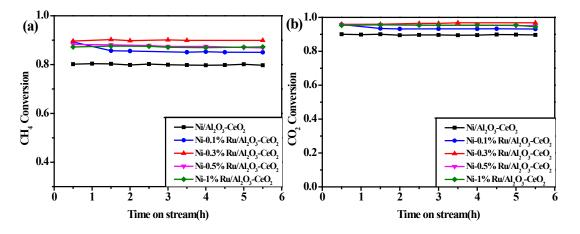
Fig. 1: Catalytic performances based on different ratios of Ru to Ni for DRM: (a)  $CH_4$  conversion, (b)  $CO_2$  conversion Reaction conditions: WHSV 27000 mL·g<sub>cat</sub><sup>-1</sup>·h<sup>-1</sup>, 1073 K.
