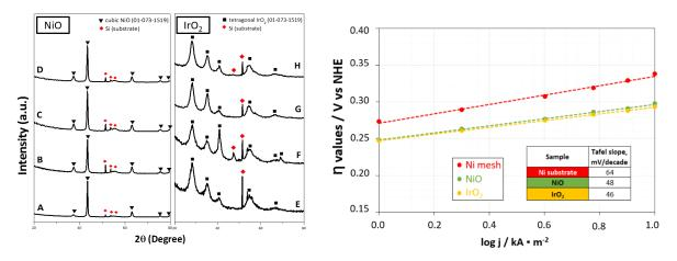
Figure 1. (a) GIXRD patterns of NiO and IrO<sub>2</sub> on Si [100]; and (b) Tafel plots of anodic overpotentials η.
