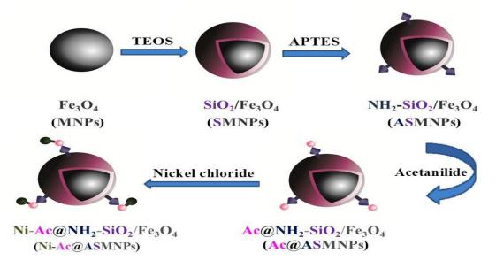
Scheme 1. Route for the synthesis of magnetic nanocatalyst with Ni as metal.
