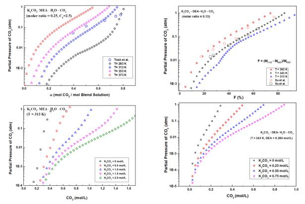
Fig 2. Solubility modeling of CO<sub>2</sub> in quaternary systems: K2CO<sub>3</sub>-MEA-H<sub>2</sub>O, K<sub>2</sub>CO<sub>3</sub>-DEA-H<sub>2</sub>O.
