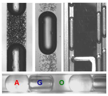
Examples of segmented flow (a) H2-water- 50 g/L Ni/SiO2 (b) G/L/beads (c) O2-cyclohexane at 30 bar, 200°C (d) Aqueous-gas(H2)-Organic (hexane) G/L/L flow.
